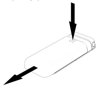
b. Pull out the isolation strip marked "PULL OUT BEFORE USE", highlighted in red below.
