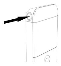
Turn the unit on by pressing and holding the power key. The unit will display the number of days left until recalibration is due, then it will display the "Wait" symbol while the sensor is heated to operating temperature.
